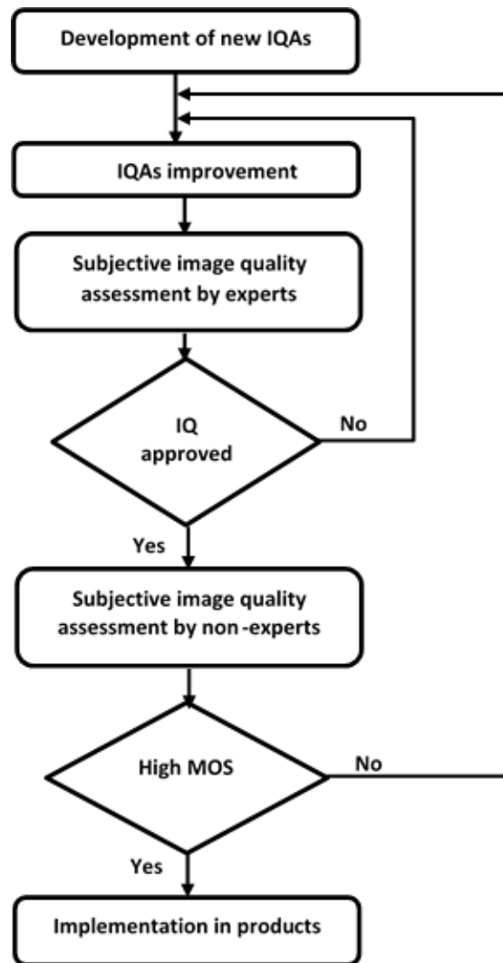
Fig.4. Actual IQ assessment process in the smartphones industry [7].
