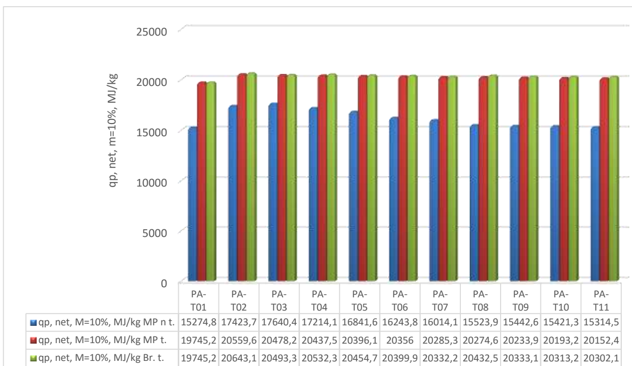
Figura 4.20. Valoarea calorifică a biobrichetelor produse din reziduuri agricole ne torefiate și torefiate: PA-T01 – paie 100%; PA-T02 – reziduuri agricole arboricole (RAA) – 100%; PA-T03 - 10w% paie+90w% RAA; PA-T04 - 15w% paie+85w% RAA; PA-T05 - 20w% paie+80w% RAA; PA-T06 - 25w% paie+75w% RAA; PA-T07 - 30w% paie+70w% RAA; PA-T08 35w% paie+65w% RAA; PA-T09 40w% paie+60w% RAA; PA-T10 - 45w% paie+55w% RAA; PA-T11 50w% paie+50w% RAA.
