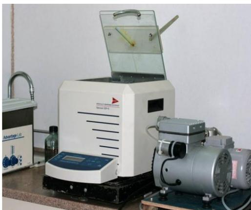
Fig. 2.10. Photo of programmable spin-coater “SGS Spincoat G3P-8”.
