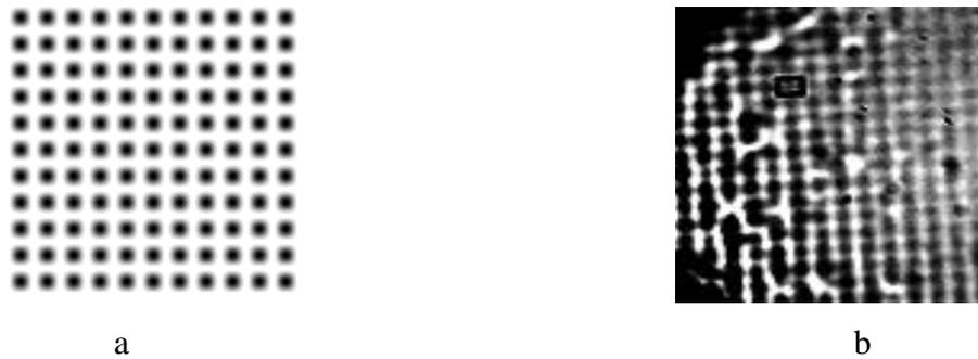
Fig. 5.17. Simulated superimposed diffraction pattern in MATLAB (a), diffraction pattern recorded on an azo-polymer film PVA: MethylRed (b).
