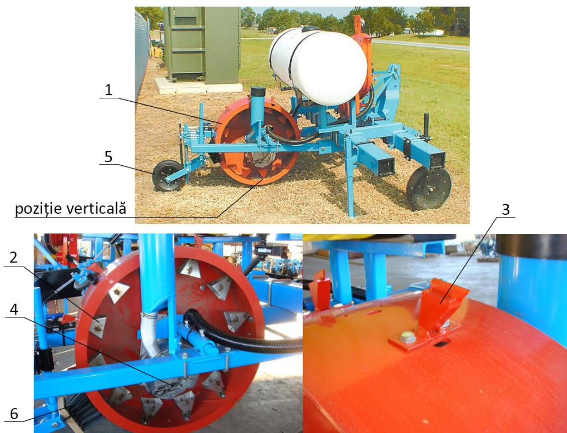
Fig. 1.7. Mașina de semănat Drum Punch Plastic Mulch Planter a firmei americane Specialty Sales Co. [50]
