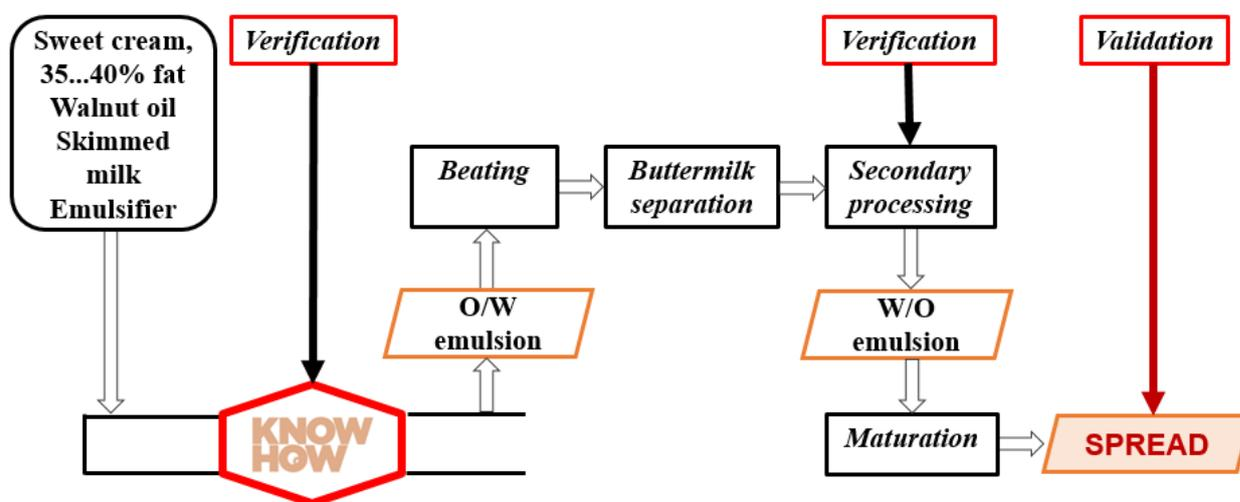
**Fig.12. General scheme of the spread manufacturing process according to the invention patent, No. 1281, 2018.09.30.**
