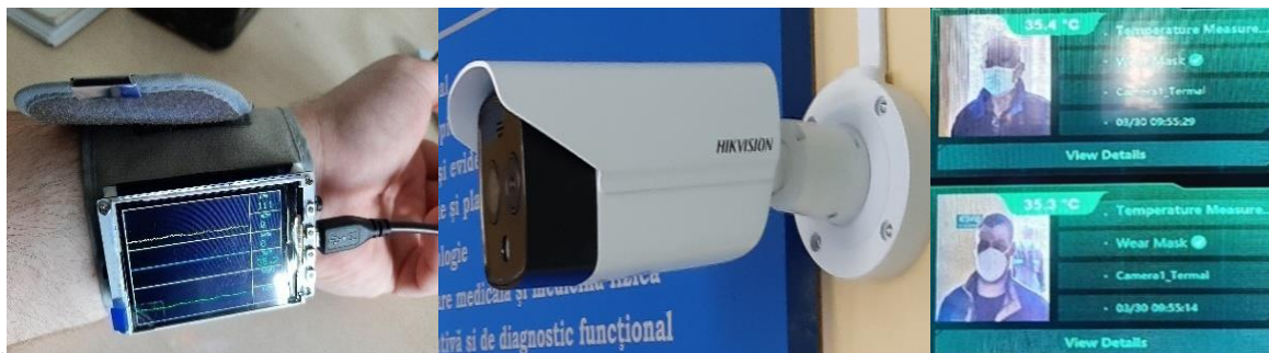
Fig. 3.8. Taking the body temperature with the help of the prototype and the thermoscanner (a) - prototype temperature determination, (b) - Hikvision thermal chamber, (c) - display of the measurement result using the thermal chamber
