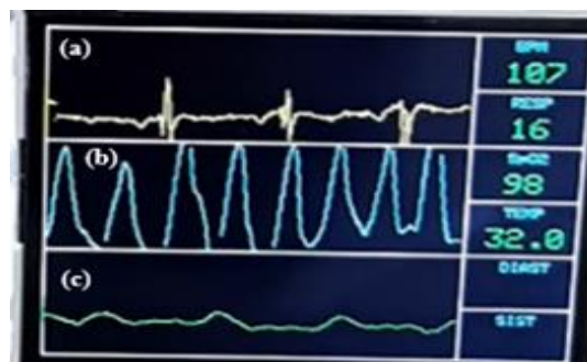
Fig. 3.5. Pneumography taken by measuring impedance
